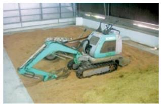
Figure 4: Mini excavator used to mix and turn the bedding
